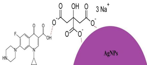
**Fig. 3.** Probable hydrogen bonding between –OH group of ciprofloxacin with –COO<sup>−</sup> groups of sodium citrate-functionalized Ag-NPs [41].
