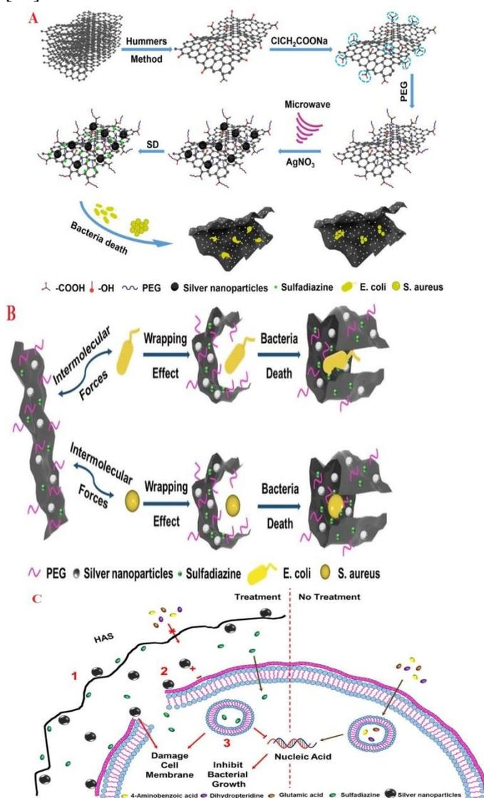
**Fig. 4.** Loading of Ag-NPs and sulfadiazine onto graphene oxide to provide hybrid multifunctional carriers with
